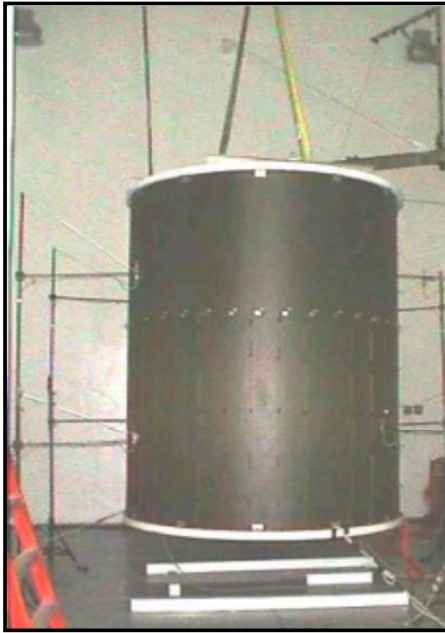
Fig. 9—Large payload shroud suspended in laboratory 3 .
